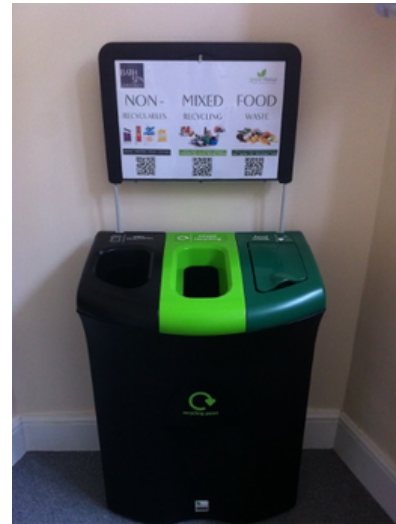
Figure 1. Example of three-stream bin for academic areas. The bin has an internal three-cassette system, which eliminates the use of bags (except for standard food waste liner) and enables rapid swap-out by our waste team.
